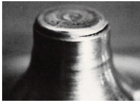
Failure due to excessive pressure at the beginning of a stroke
